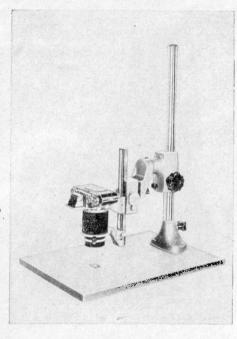
the little fixing screw (at the lower end of the column head) secures it. After loosening the big screw (opposite the black rack-and-pinion knob), the front part of the column head can be turned, and when fastened again, fixed in every desirable position.
