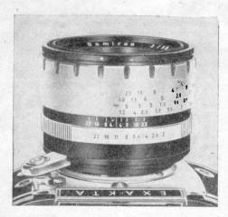
When using infra-red film, first focus according to the ground glass too. Then adjust the subject distance indicated (infinity sign, numbers of metres or feet) from the red index dot to the red point (infra-red point) to the left. Thus the image produced by the invisible infra-red rays,
